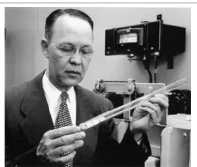
Calvin S. Fuller at work diffusing boron into silicon to create the world's first solar cell
